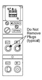
To set the Zero/Span enter the calibration screen of the tester. Select the Adjust Regulator button. Use the +++ button (15-20times) to drive the regulator up to full scale. Adjust the span screw (above the word SPAN) until the pressure output pressure is 1% higher than full scale (example 60.6 for a 60psi unit). Press the zero button to send the regulator output to zero pressure. Adjust the ZERO screw until the pressure output is 0.010psi.
